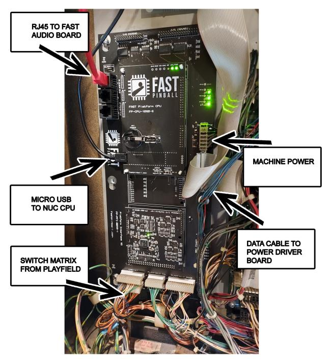
FAST WPC-95 CONTROLLER REV2 (INSTALLED)
