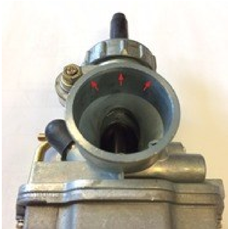
Idle Pilot Jet - Stock, Unaltered #32, .0130" No-go
