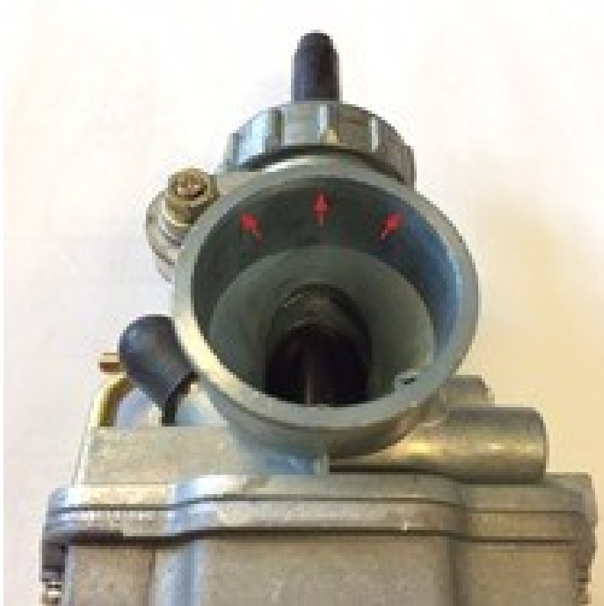
Idle Pilot Jet - Stock Unaltered #32, .0130" No-go
