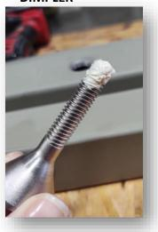
3. SCREW IMPACT DOOR DIMPLER BY HAND 1-2 TURNS
