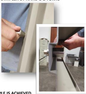
4. TIGHTEN DIMPLER WITH CORDLESS TOOL OR ALLEN WRENCH UNTIL DESIRED DIMPLE IS ACHIEVED
