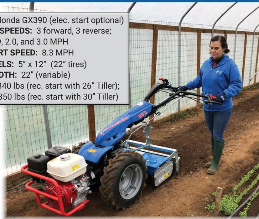
The difference between Models 852 and 853 is simple: The transport speed is only accessible in rear-mount (Tiller) mode on the 853. On the 852, the transport speed is only accessible in front-mount (Mower) mode. Model 852 is the choice for users who will primarily be using their tractor for mowing and snow removal.
