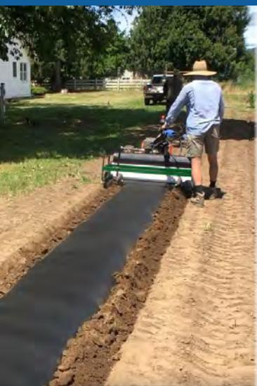
With an updated design, the Plastic Mulch Layer now supports both 36" & 48" plastic rolls. It will flat-lay 36" plastic, leaving approx. 26" exposed. It will also flat-lay 48" rolls, leaving approx. 38" exposed. Raised beds can be covered using 48" rolls, provided they are approx. 30" wide and no more than 3" high. A prerequisite is that the soil needs to be well-worked, dry, and level.
