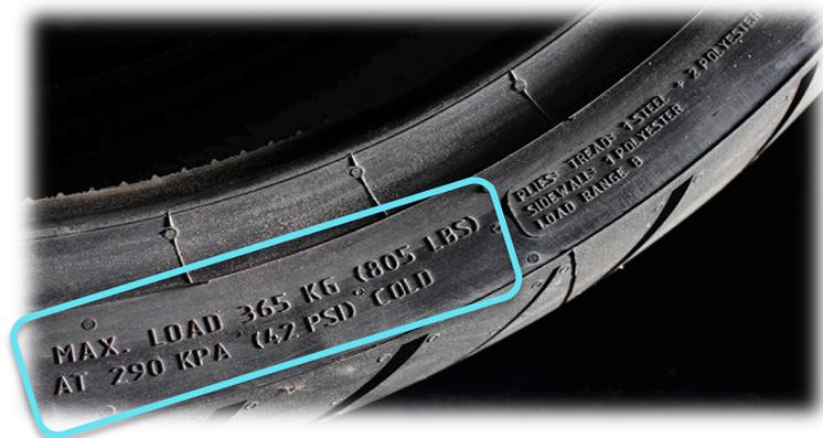
The maximum load – here it's 365kg – is the most the tyre can support at a standardised pressure – in this case 42psi. This isn't necessarily the pressure recommended for your bike, so check your owners' manual or the tyre manufacturer's fitment guide.
