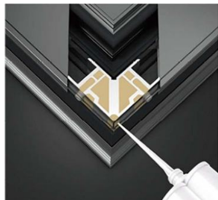
Corner Injection Molding Process
