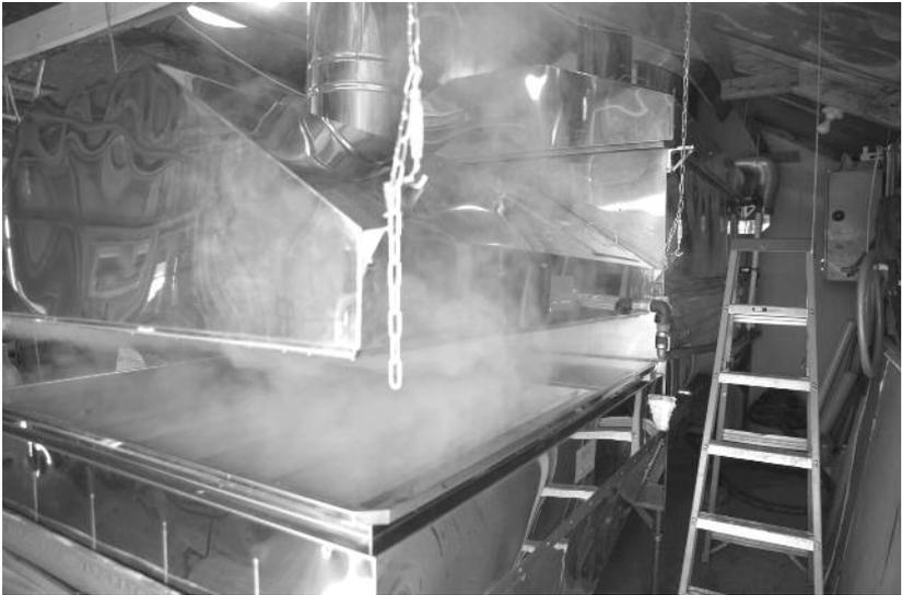
*Sap boiling in an evaporator.*
