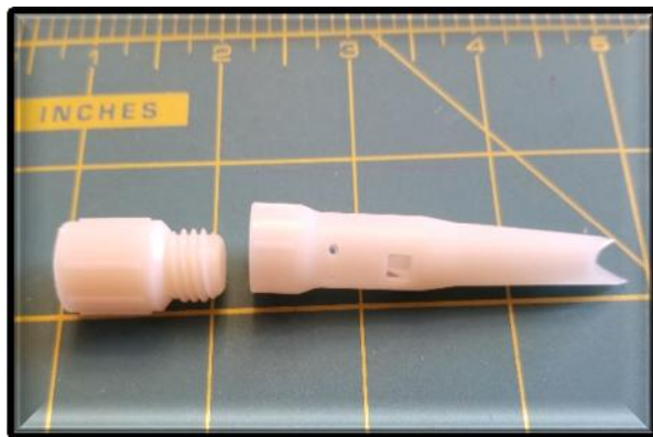
Pre-assembled dart tip and base can be separated after sample acquisition or bagged and frozen intact
