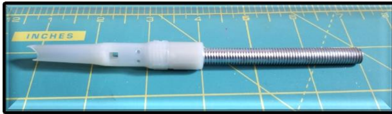
TISSUEGRAB™ Biopsy Dart include dart tip and base mounted to an M8 bolt.
