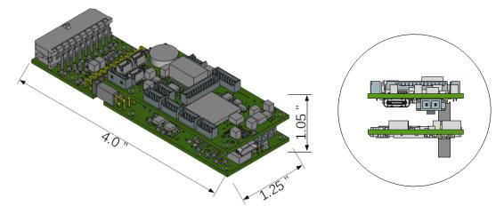
**16-channel stacking example:** The header system on the A2D board makes it possible to stack multiple A2D boards with a single digital board; identical or different AcSense-IB boards may be used for input into the two A2D systems. Image to the right shows fit of 16ch assembly in 2" diameter tube. NOTE: height **includes** bottom header on bottom AcSense-ADM-A2D; this part comes populated on the standard board but may be removed if unused.
