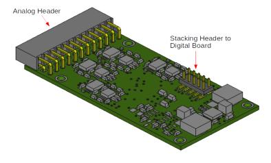
AcSense-ADM-A2D: Analog header to connect to AcSense-IB-XXX; stacking header to connect to AcSense-ADM-Digital. Powered from stacking header.
