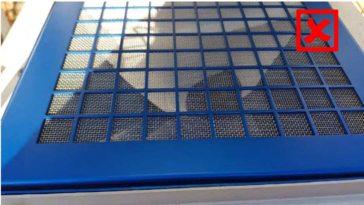
Figure 9. An example of an incorrectly installed HVAS filter paper.
