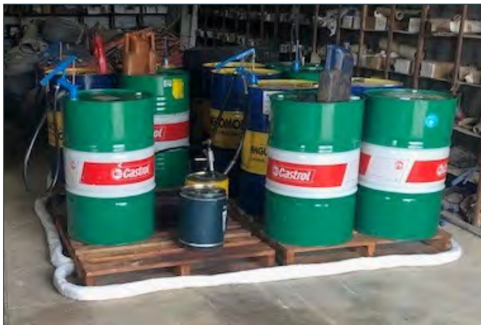
Photoplate 1. Roll Bunds Installed in Workshop
