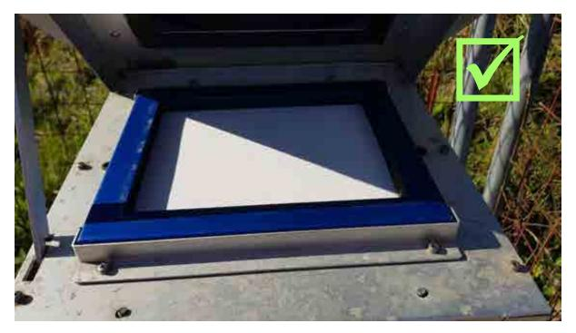
Figure 8. A correctly installed HVAS filter paper
