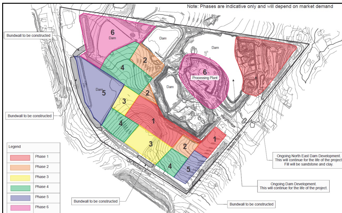
Figure 2.13: Plan showing the proposed modified sequence of extraction. A full copy of this plan, together with a plan of each Phase, is at Appendix 10 .
