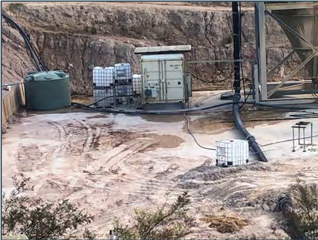
Empty IBC's in Chemical Storage Area
