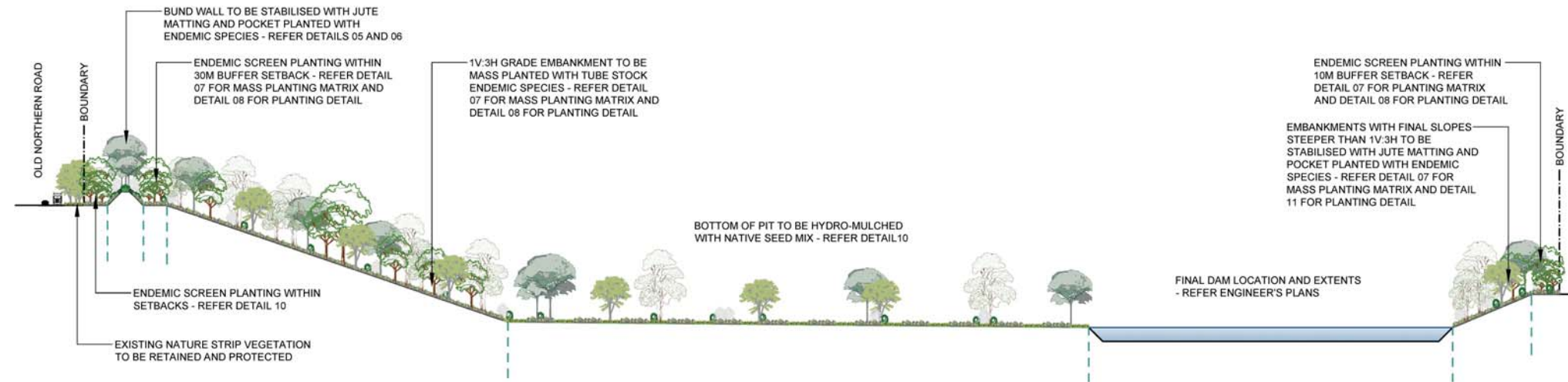
SECTION AA: FINAL REHABILITATION OF SITE SCALE 1:1000
