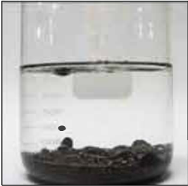
Demonstrates the immediate release of oil from sand using an 80/20 blend of SC-1000 and SC-SuperSolv at a 5% solution in water.
