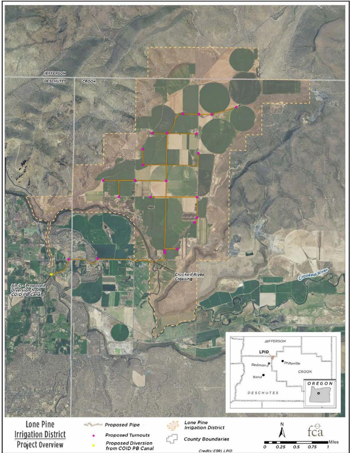
Figure 11. Lone Pine Irrigation District’s Piping and Pressurization Alternative
