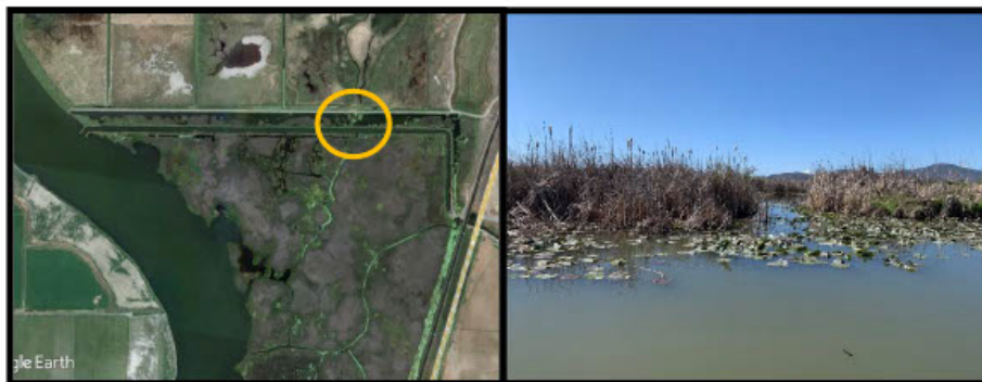
Figure 4-d. Example of a break in the southern levee of the North Canal
