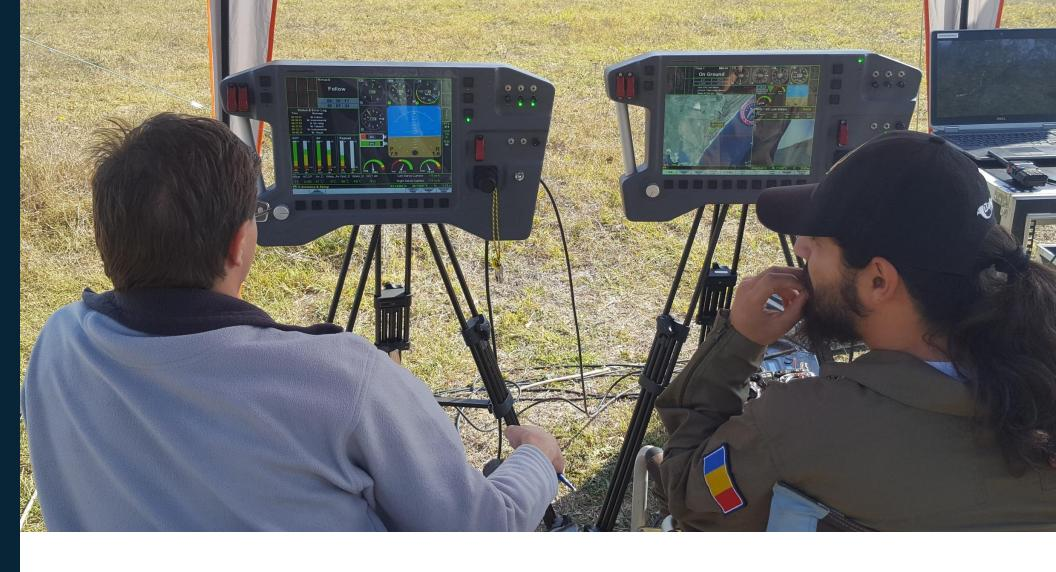
At the Ground Data Terminal multiple Ground Control Stations can be connected over an IP network. With the help of an appropriate infrastructure, such a connection can be made even via the Internet. Ground control station is available both as an embedded solution and as an application on the PC. Integration with Command-and-Control Centers is therefore particularly easy.
