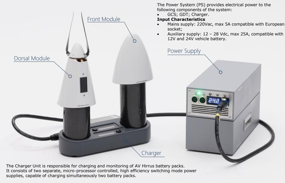
The Charger Unit is meant to be powered up mainly by the Power System. But the wide input voltage range allows charging from a vehicle power systems (12V or 24V) or external power supplies, with a maximum input voltage of 30V.
