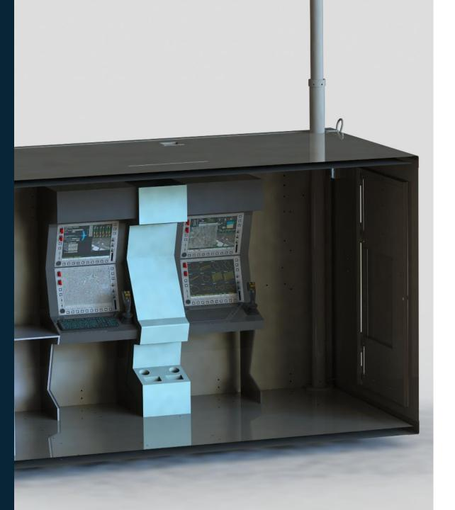
The concept is based on MFD (Multi Functional Display) modules designed for ease of operation. The Ground Control System (GCS) contains all the necessary capabilities required for managing the entire system:
