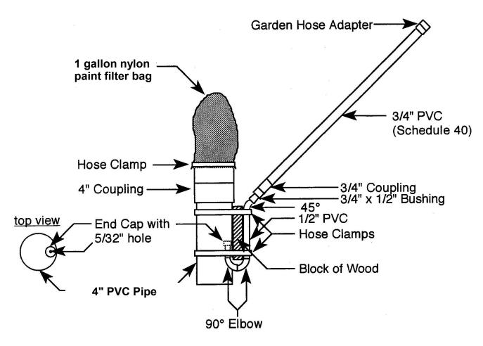
This pond vacuum does an excellent job of sucking up leaves and other vegetation from the bottom of your pond. The bottom end of the 4" pipe is open to allow debris to be pulled into the pipe and then into the nylon paint filter bag by the force of the water rushing out of the 5/32" hole. The coupling and filter bag assembly is just pushed onto the 4" pipe. When you are done vacuuming, pull off the coupling and
