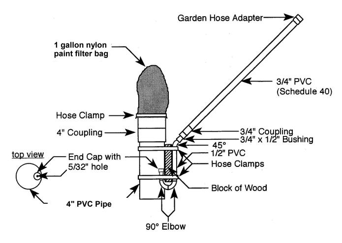
This pond vacuum does an excellent job of sucking up leaves and other vegetation from the bottom of your pond. The bottom end of the 4" pipe is open to allow debris to be pulled into the pipe and then into the nylon paint filter bag by the force of the water rushing out of the 5/32" hole. The coupling and filter bag assembly is just pushed onto the 4" pipe. When you are done vacuuming, pull off the coupling and rinse out the filter bag. All other PVC fittings are glued together.
