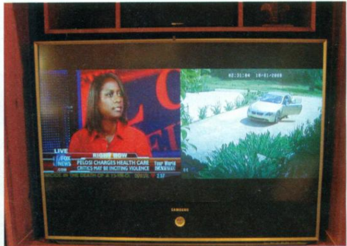
FIGURE 2 A popular application for sensors and cameras is when a car or person approaches the home the system engages the TV's picture-in-picture to display the appropriate camera on the split screen for 15 seconds.
