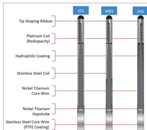
Figure 6. Innomed Coronary Guidewire Inno-Pathwire Design Structures. STS=light support; MDS=moderate support; EXS=extra support.
