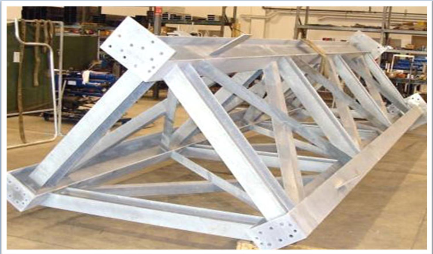
HOT DIP GALVANIZED STEEL STRUCTURE
