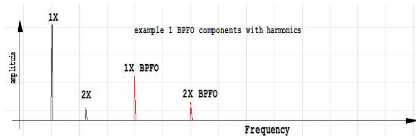
Outer race damage spectrum with harmonics.
