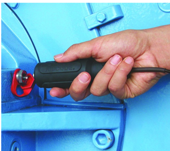
Connect the VIBCODE sensor to the VIBCODE measurement location.
