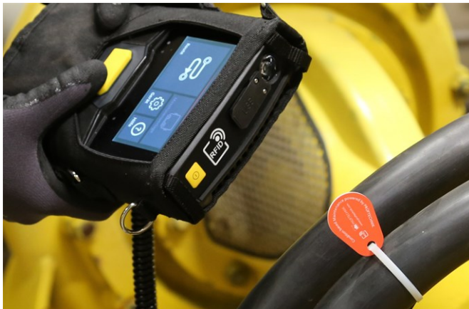
The RFID reader captures the code of the transponder without contact.
