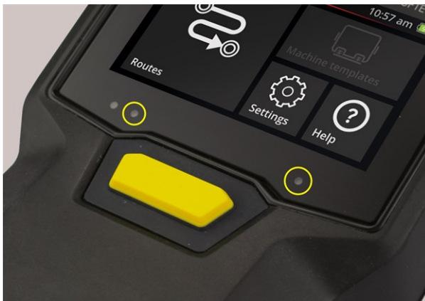
Two inlet openings for ambient light sensor.
