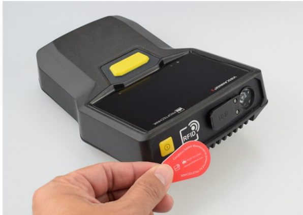
Identifying measurement locations using RFID technology (ISO 14443a and ISO 15693).
