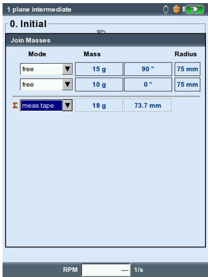
Left: Result for measuring tape correction mode
