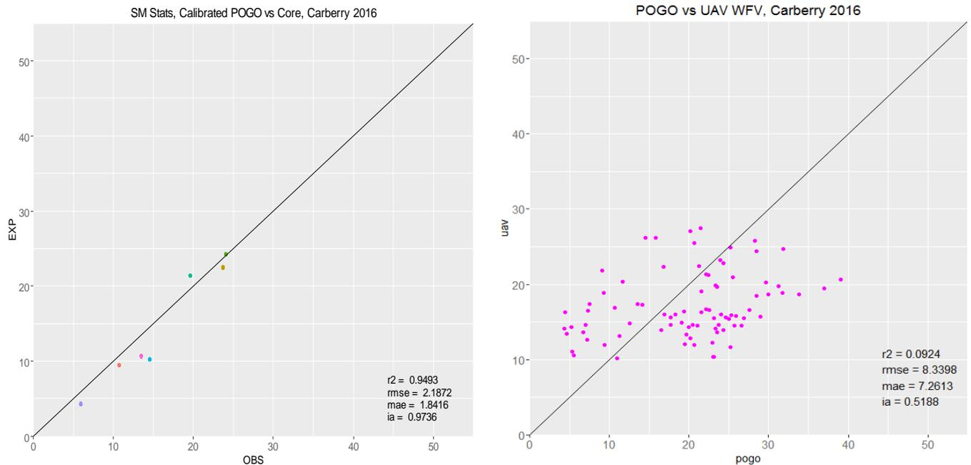
**Figure 4.** Soil moisture plot generated using the calibrated POGO data and core samples from the plots in Carberry, 2016 with outliers removed (left). OBS values correspond to VWC calculations from core samples while EXP values correspond to the POGO data. POGO vs UAV plot using all overlapping data captured during the 2016 Carberry campaign (right).
