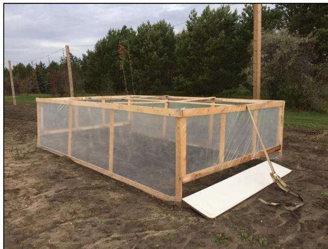
**Figure 2.** Rectangular heat chamber test design – built to span three potato rows and installed and removed multiple times in season.
