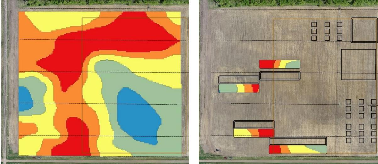
**Figure 1.** VRI prescription designed for entire western third of the CMCDC Offsite, using topography and soil test results (left image). From this map, four paired comparison plots were identified (right image), showing the VRI (multi-colored rectangles) vs. URI (blank rectangles bordering on the N or S of the colored plots) plots. Multiple benchmark sampling points were established in each of the plots, within the various management zones.
