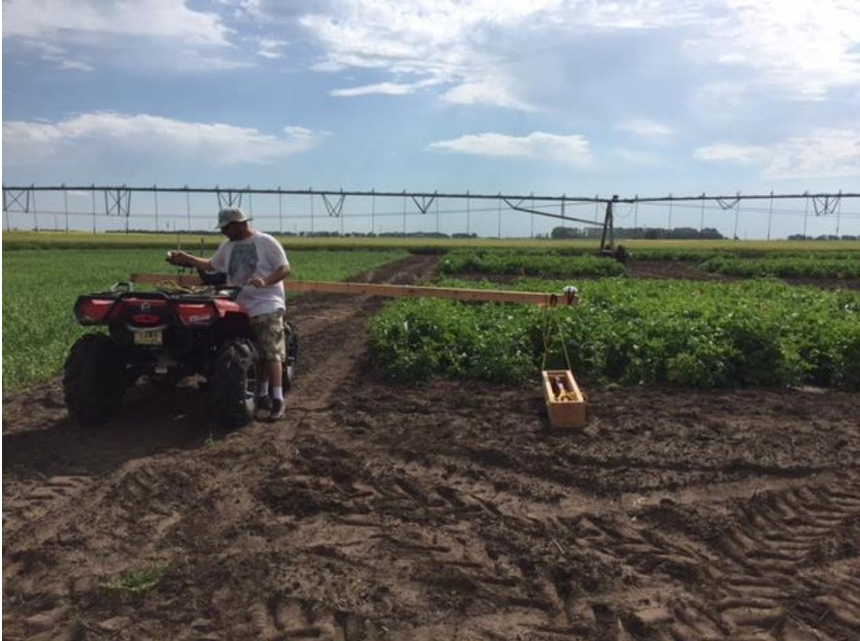
**Figure 1.** The Em38 in a cradle, offset from the ATV, with a GPS receiver mounted above it, to be pulled through the furrow between two potato rows. The cradle rides on the surface of the soil.
