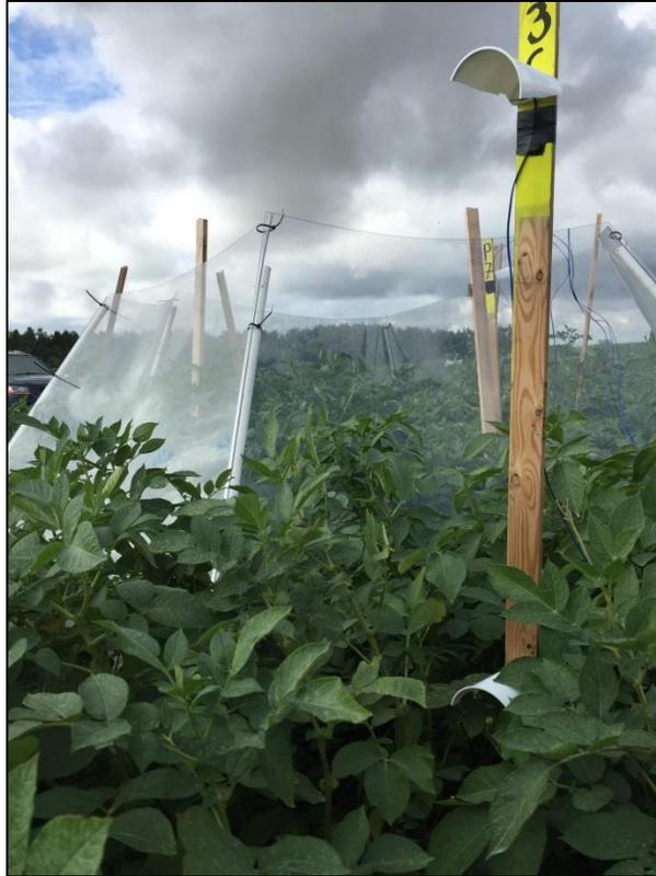
**Figure 1.** Hexagonal Plexiglas heat chamber design installed in a potato plot. Themocouple sensors installed on stakes inside and outside the chambers to monitor canopy temperatures.
