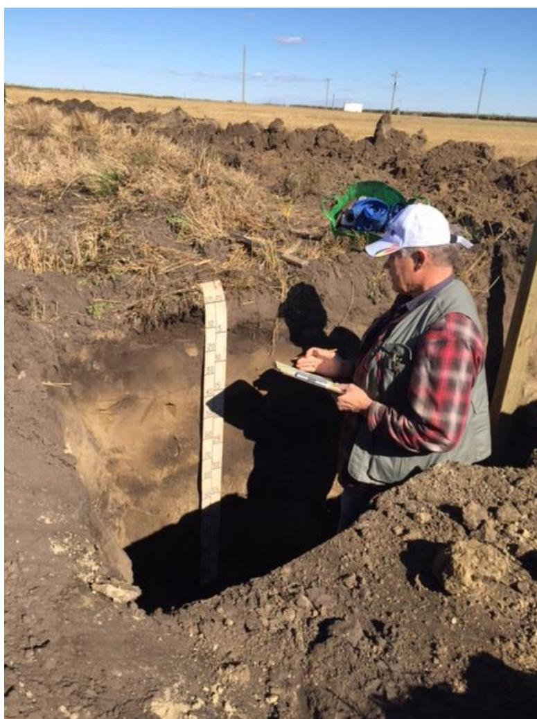
**Figure 1.** Soil pedologist taking notes on soil profile and characteristics at one of three soil pits dug at CMCDC-Carberry
