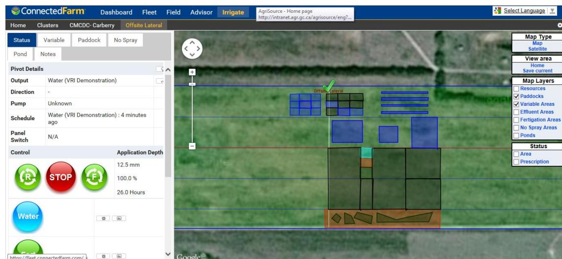
**Figure 2.** Screenshot of Trimble Connected Farm Irrigate-IQ™ system used for control and monitoring of the CMCDC VRI system.
