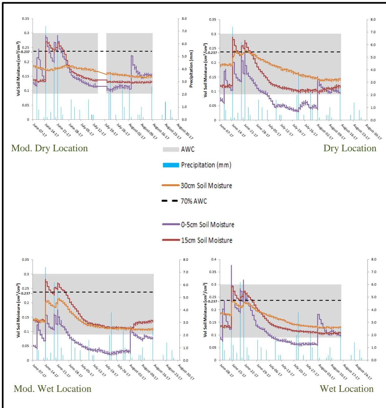
**Figure 2.** Field 1 soil moisture and precipitation June 8-Aug 15 at the four installed soil moisture stations. Each chart is data from a different location in the field.
