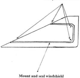
Mount and seal windshield using 3M 4200 adhesive or equivalent
