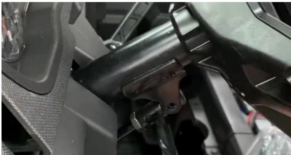
Lower Bolt Removed
