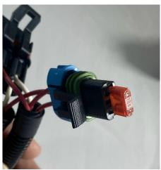
2.6. Check the pulse connector and ensure it is seated properly into the pulse power bar or if on a model without a pulse power bar, ensure the adapter is getting proper power.
