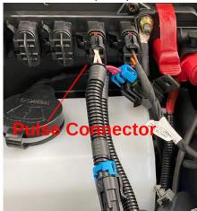
2.7. Check the main harness connection to the Base Unit connector.
