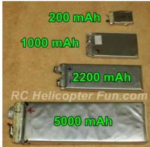
*RC LiPo Battery Capacity Cell Size Comparison*
