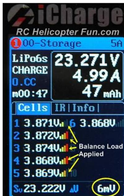
Some chargers will actually show you the balancing process in real time as shown in this photo while charging a 6-cell LiPo battery with my [iCharger 4010 Duo](#).
