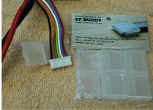
I started using [these AB clips](#) recently and they work so well to prevent the wires from being pulled out of the plugs because you can now actually grip the plug. They are super easy to install as you can see in the picture here. Just place the JST-XH plug in the unfolded AB clip and fold the clip closed - done!
