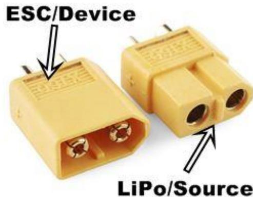
*Typical RC LiPo Battery Connector*
