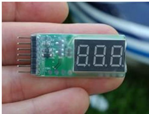
I for instance use these little inexpensive LiPo battery monitors after most flights to gauge my flight times to ensure I'm not over discharging my packs much past 80%. These ones I use work with 2S to 6S LiPo packs.
