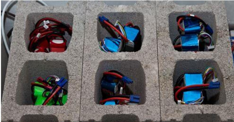
*RC LiPo Batteries Safely Stored In Concrete Blocks*
