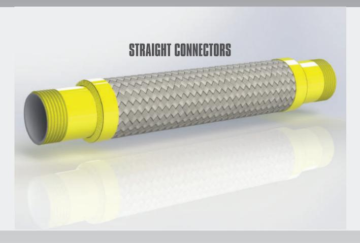
EFP CSA rated flex connectors are designed for use as a connector in medium pressure natural gas applications in the United States and Canada. They are built to length and come with either carbon steel or stainless steel Sch40 male NPT ends or beveled weld ends. Every assembly is pressure tested and is rated to 150 psig.
