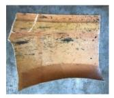
1. Sand/clean at least a ½" On both sides of the crack and on both sides of the part
