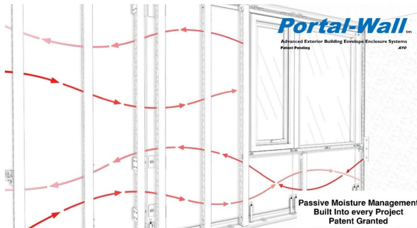
Visualization of the proposed air flow through the Portal Wall exterior wall cavity
