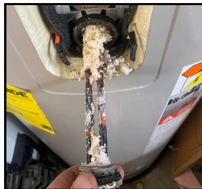
Severely Scaled Heating Element
