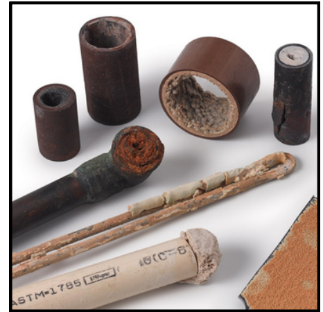
Scale buildup in various plumbing pipes (before Superior installed)
