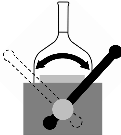
Figure 2 – Tightening and loosening range of motion in vise
