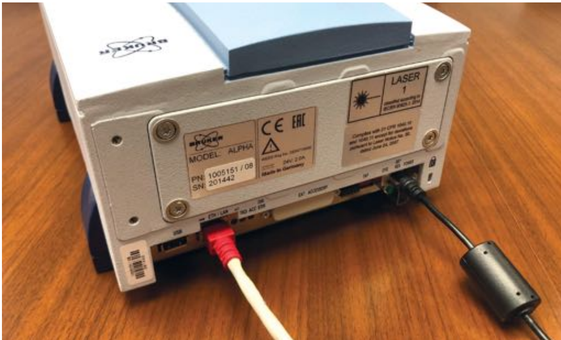
Figure 3. FTIR ethernet port (left) and power port (right).
