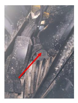
• Feed the open plug ends of the cage harness up through the bottom of the driver side front cage pillar. Use the slots in the side of the pillar to help run the wire up to the top exit hole.
