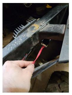
• Run the light harness along the OEM tail light harness to the rear of the machine by the bed bracket and run the split to the proper side of the machine. Connect the bullet connectors to the lights. Attach the light harness to the OEM wiring using the supplied zip ties. In the location by the exhaust wrap the wires with the supplied heat tape.
