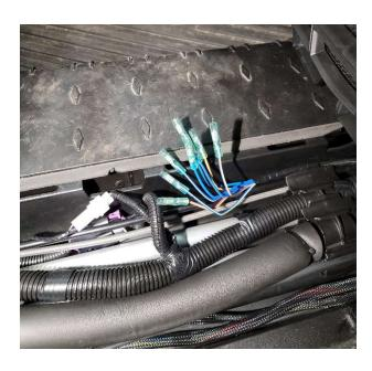
• Remove the dash switch panel by gently pulling the bottom side toward you. Then the top should unhook to give you access to the other end of the OEM bullet connections.
