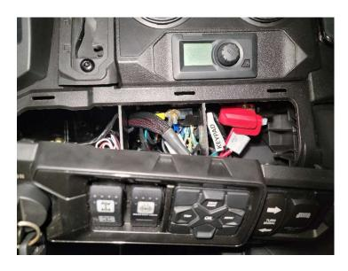
• Attach the bullet electrical connectors to the OEM harness bullet connectors under the dash. Be sure the attach the red and black wires to the same color wires as below in the floor.
