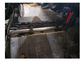
• Run main wire through the bottom of the firewall in the rear and up along the wires to the top of the gas tank
