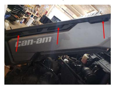
Remove the stock tail lights by removing the connector and then the 2 bolts on the inside of the bed where tail gate folds up. Bolts will use a 10mm socket. Lift up on the top part of the connector to remove the plug.
