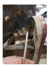
• Remove the two metal clips from the OEM tail lights by lifting up on the inside of the clip and sliding it off. Make sure the clip inner looks like the picture below so it latches to the new light correctly.
