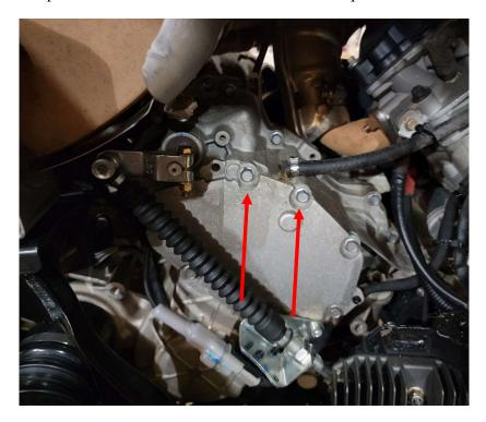
• The two holes in the switch bracket will line up and mount to the holes in the transmission where the bolts were removed. Reuse the bolts that were taken out to attach the bracket to the transmission. These should be tightened down to 90in/lbs.
