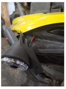
With light pressure hold the housing in place and secure using the supplied screws. Each housing
