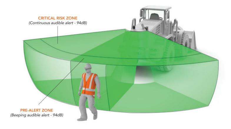
Multiple sensors can be used to achieve a 120° field of view. The detection area can be configured with two alert zones, a pre-alert zone (beeping audible alert), and the critical risk zone (continuous audible alert). The pre-alert gives the operator and pedestrian time to modify their behavior before they enter the critical risk zone.
