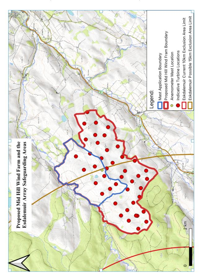
Eskdalemuir Possible 15km Exclusion Area Limit Eskdalemuir Current 10km Exclusion Area Limit Proposed Mid Hill Wind Fram Boundary Indicative Turbine Locations Anemometer Mast Location Mast Application Boundary egend: Proposed Mid Hill Wind Farm (2025) and the Esdalemuir Array Safeguarding Areas
