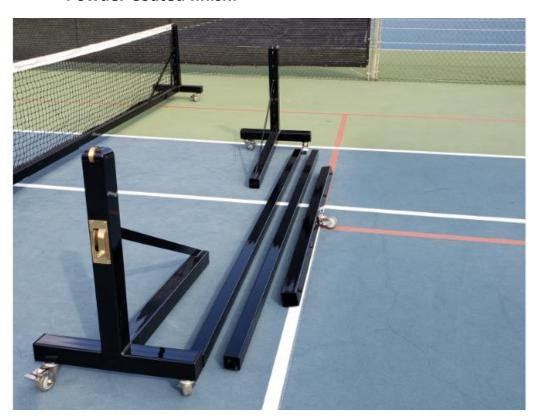
Step 2: Install the four end post wheels that have the step-down brakes.
