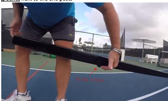
• Carefully slide them together until the welded steel stop, rests against the end post section.
